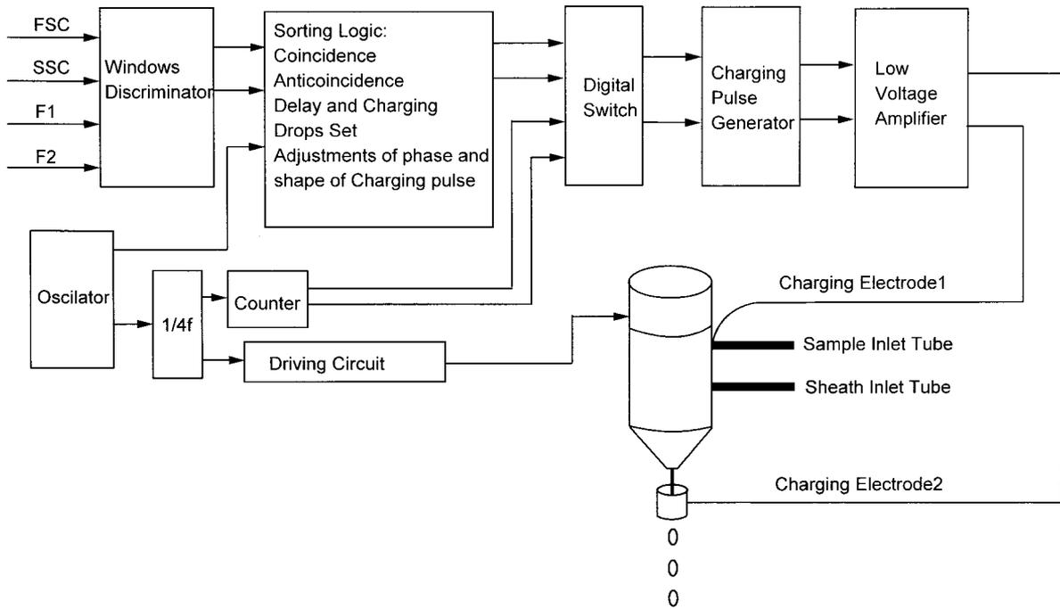
FIG. 1. Schematic diagram of signal-processing circuit.
