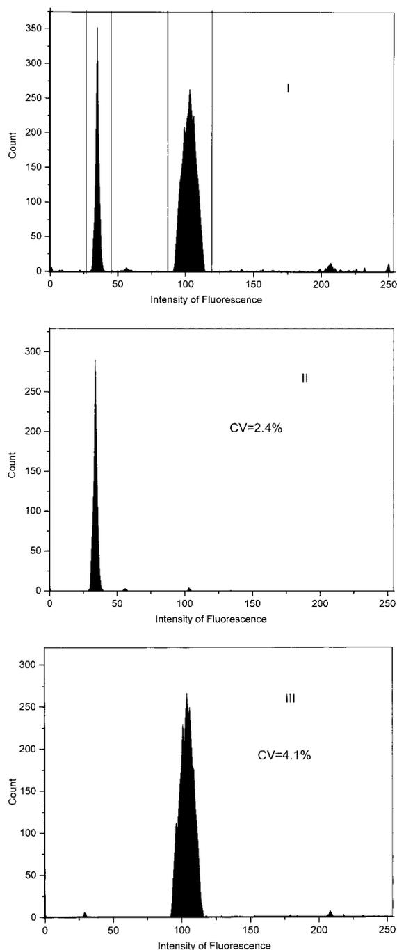
FIG. 3. Fluorescence distribution histograms. **I:** Mixture of plastic microspheres and chicken red blood cells. **II:** Separated fluorescent microspheres with purity of 99.2%. **III:** Separated chicken red blood cells with purity of 98.6%.
