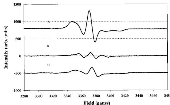
**Figure 4.** Hydration effects on ESR signals of potato cell walls containing TEMPO. (A) Dried sample; (B) containing 27% water; (C) after drying over P<sub>2</sub>O<sub>5</sub> under vacuum.
