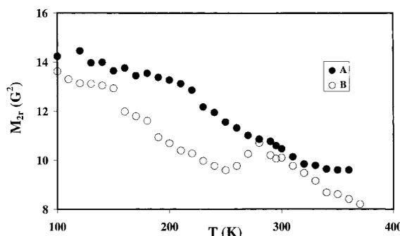
**Figure 7.** Proton residual second moment data for CWC. (A) Dry sample; (B) containing 21% D<sub>2</sub>O.
