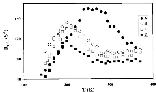
**Figure 6.** Proton spin–lattice relaxation rate in the rotating frame for CWC. (A) Dry sample, spin-locking field 40 kHz; (B) containing 21% D<sub>2</sub>O, spin-locking field 42 kHz; (C) containing 21% D<sub>2</sub>O, spin-locking field 67 kHz; (D) containing 21% D<sub>2</sub>O, spin-locking field 100 kHz.
