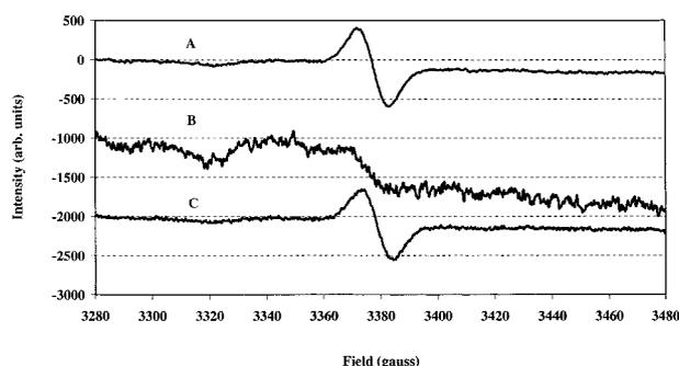
**Figure 3.** Hydration effects on ESR signals of cell wall materials of Chinese water chestnut. (A) Dry sample (receiver gain, 4000); (B) containing 13% water (receiver gain, 10 000); (C) after drying over P<sub>2</sub>O<sub>5</sub> under vacuum (receiver gain, 4000).
