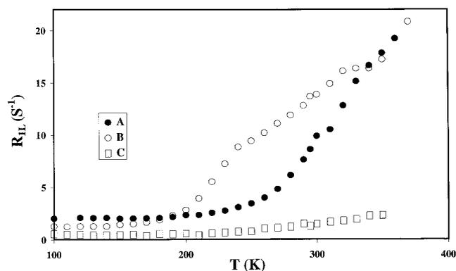
**Figure 5.** Proton spin–lattice relaxation rate in the laboratory frame for D<sub>2</sub>O exchanged CWC and PB. (A) Dry sample; (B) containing 21% D<sub>2</sub>O; (C) dry PB.
