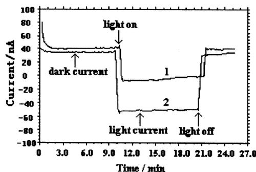
Fig. 1. Photoelectric current of rat cerebellar granule cells responding to white light. 1) Photoelectric current of ITO without cells; 2) Photoelectric current of ITO with cells.
