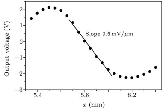
**Fig. 2.** Output signal versus displacement  $x$  of bead image with respect to QD. The dots represent the output voltages acquired by moving the QD with a step of  $50\ \mu\text{m}$  in the  $x$  direction. A linear fit of the chosen range gives the ratio of output voltage to displacement of the bead image.
