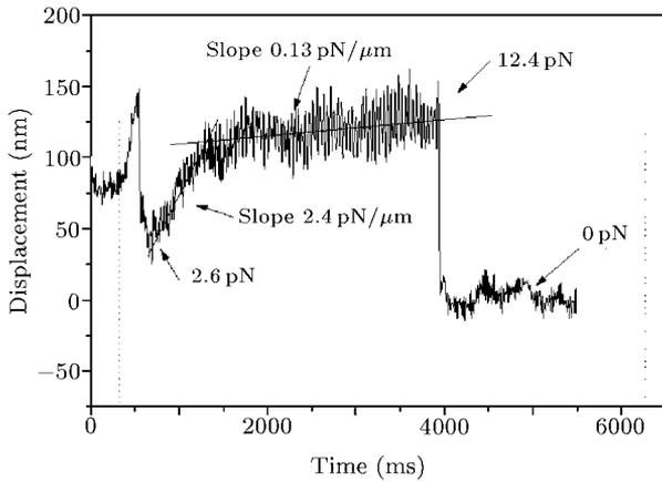
**Fig. 3.** Displacement of trapped bead during the membrane tether formation and break.
