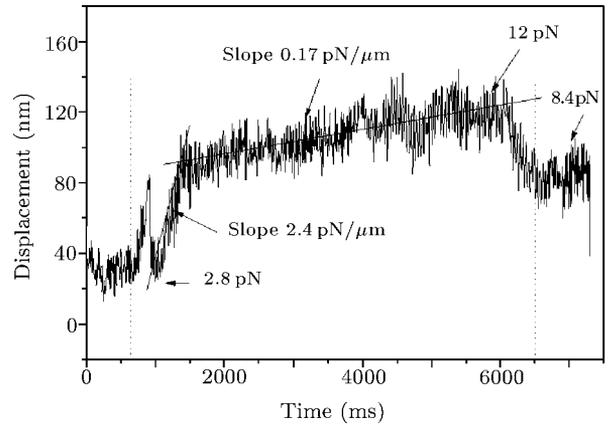
**Fig. 4.** Displacement of a trapped bead before and after stopping movement of the stage. The dynamic and static tether forces are calculated by the displacement of the bead.
