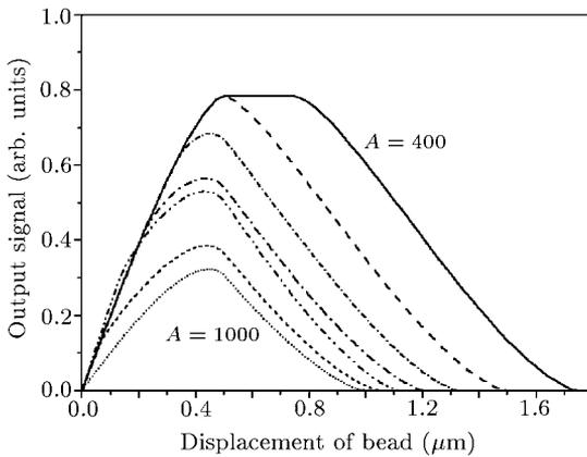
**Fig. 1.** Dependence of output signal on the bead displacement under different magnifications from  $A = 400$  to  $A = 1000$ .
