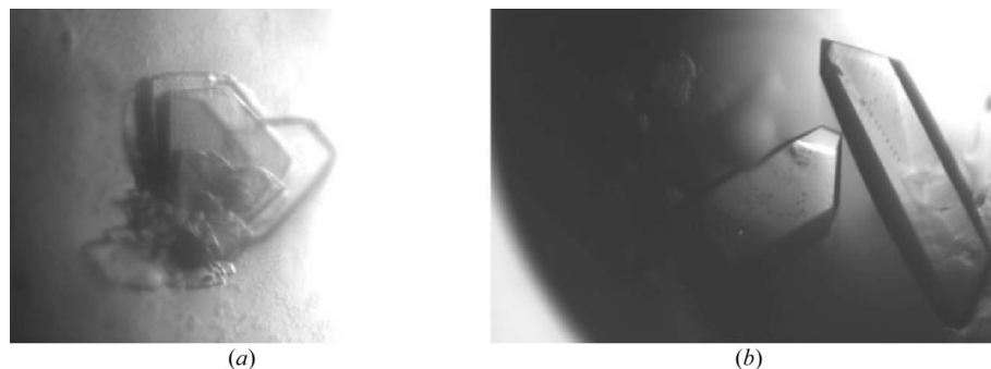
Figure 1 Two crystal forms of SPE10. (a) A typical crystal obtained from 10% (v/v) PEG 8000, 0.1 M MES pH 6.5, 0.2 M zinc acetate. (b) Crystals grown in 35% (v/v) PEG 8000, 0.1 M HEPES pH 7.0. The diffraction data were finally collected using crystal form B .
