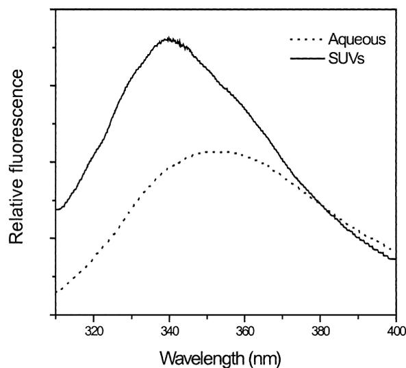
Fig. 4. Fluorescence emission spectra of peptide C21w in aqueous solution (dotted line) and following its interaction with soybean phospholipid SUVs (solid line). The peptide concentration was  $2 \mu\text{mol/L}$  and that of SUVs was  $200 \mu\text{mol Pi/L}$ . Excitation wavelength was set at 295 nm, and the emission spectra were recorded from 310 nm to 400 nm with bandwidths of 5 nm for both excitation and emission.
