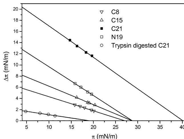
Fig. 2. Interaction of synthesized peptides with soybean phospholipid monolayer. Displayed is the  $\Delta\pi$ - $\pi$  plot of surface pressure changes after injection of synthesized peptides (2.5  $\mu\text{g/ml}$ ) underneath soybean phospholipid monolayer at different initial surface pressures. The limiting surface pressures of peptides N19, C8, C15 and C21 were 28.78, 27.09, 28.74 and 40.13 mN/m, respectively, and that of trypsin-digested peptide C21 was 19.13 mN/m.
