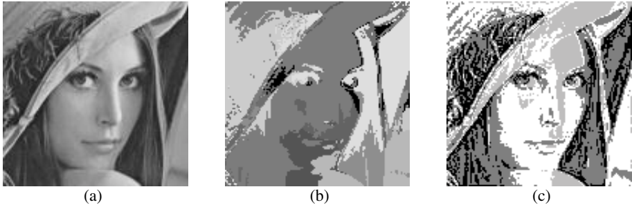
Fig. 1. (a) original image; (b) segmentation results by using the MBNN. The number of iterations is 5. k_0=40 , k=20 ; (c) segmentation results by using the MRF-MBNN. The number of iterations is 3. k_0=40 , k=4
