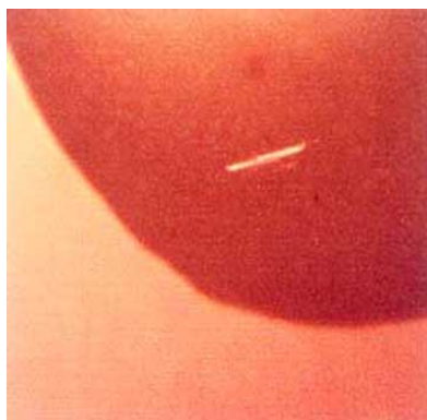
Figure 1. Typical crystal of EoCen grown using the hanging-drop method in 20% PEG 3350, 0.2 M NaCl.
