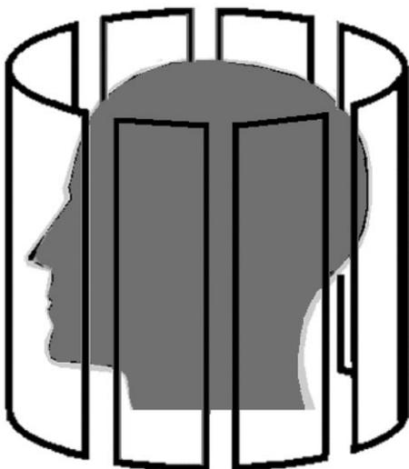
FIG. 2. Sketch of the 8-element head coil for simulations of radial SENSE imaging.
