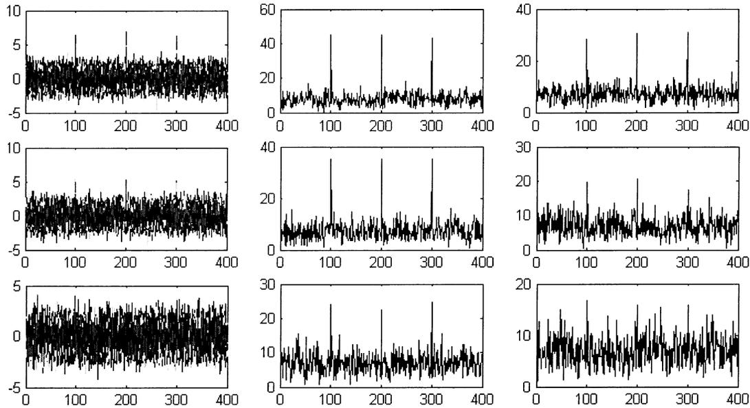
Fig. 5. Result of DSD. (ai) Simulation data with various SNR. (bi) Result of DSD with  $\beta = 3$  and  $L = 3$ . (ci) Result of DSD with  $\beta = 0$  and  $L = 1$  (PCA). The horizontal axis is the number of voxels, the vertical axis is the intensity value of the signal. Where  $i = 1$  with SNR = 1.5 dB,  $i = 2$  with SNR = 1.0 dB, and  $i = 3$  with SNR = 0.7 dB.
