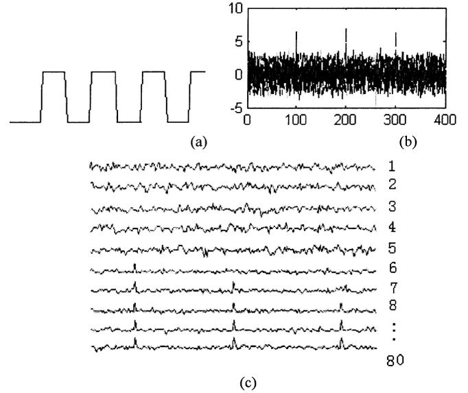
Fig. 1. Simulation data. (a) Block signal simulating a fMRI stimulus pattern; (b) An fMRI dataset with three activation locations; the horizontal-axis is the order number of voxel, the vertical axis is the intensity value of the signal. (c) The simulated fMRI dataset with three asynchronous activations in Gaussian noisy background with different delay-times.
