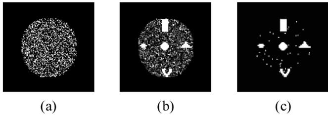
Fig. 4. Result of NC. (a) Synthetic pattern at one single time point; (b) distribution of the NC coefficient; (c) imaging result of NC with a threshold 0.3.
