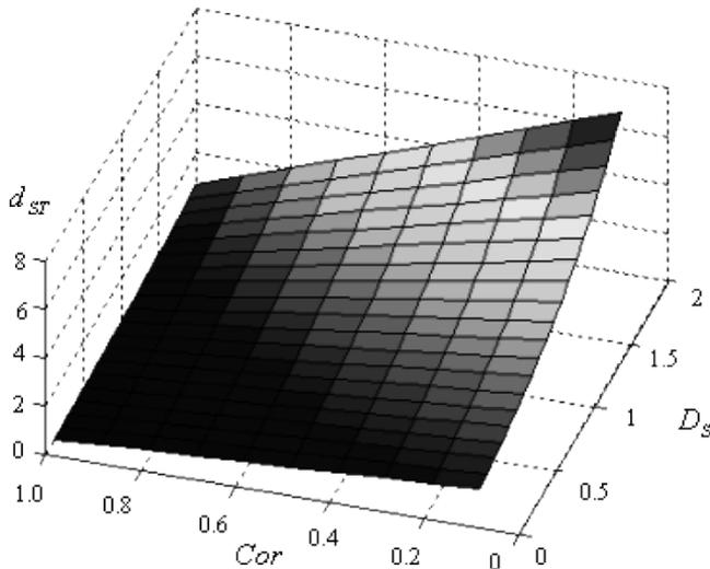
Fig. 2. Spatio-temporal distance measure. The vertical axis is the distance measure  $d_{ST}$ , the two lateral axis are the temporal  $Cor$  between two voxels and the L1 norm spatial distance  $D_S$  of two voxels.
