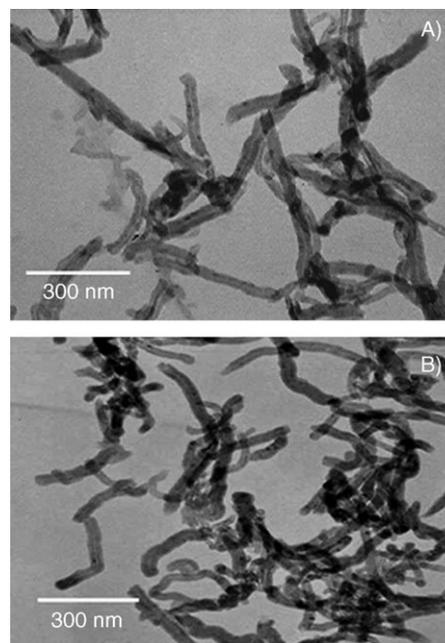
Figure 1. TEM images of A) NH<sub>2</sub>-MWCNTs and B) NH<sub>2</sub>-MWCNT-DNA.
