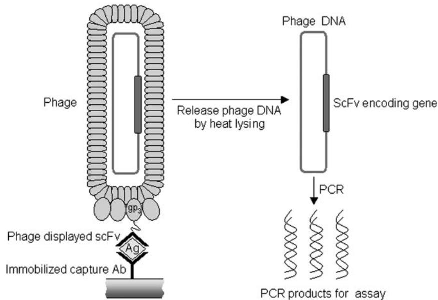
**Figure 1.** Schematic diagram of phage display mediated IPCR.
