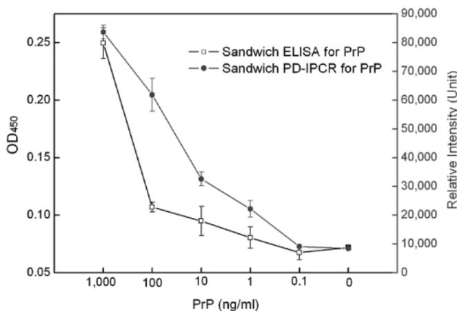
**Figure 5.** Detection sensitivity of sandwich PD-IPCR and sandwich ELISA for PrP. The amplification band of PD-IPCR was quantified by a computer assisted image analyzer. The color development in ELISA was achieved with HRP-labeled anti-M13 monoclonal conjugate secondary antibody and TMB substrate. Average values of three independent experiments are given.
