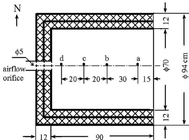
Fig. 1. Sectional drawing of the HMF space used in the present study. The natural GMF was substantially shielded in the cylindrical chamber, consisting of three laminae of Permalloy plates (1 mm thickness) and intermediate insulation fillers. The residual magnetic field intensity, measured with a fluxgate magnetometer, was 2.8, 0.1, 0.048, and  $0.022 \mu\text{T}$  at positions a–d, respectively. The hamsters were held in cages placed between b and d. All dimensions in cm.
