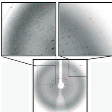
**Fig. 3.** A typical X-ray diffraction pattern from a native mitochondrial complex II crystal.
