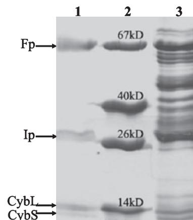
**Fig. 1.** SDS-PAGE analysis of the crystallization preparation and the crystal of complex II. Lane 1, crystals of complex II. Lane 2, molecular weight markers. Lane 3, crystallization preparation of complex II. The four subunits of complex II are labeled on the left, and the positions of molecular weight standards are indicated on lane 2.
