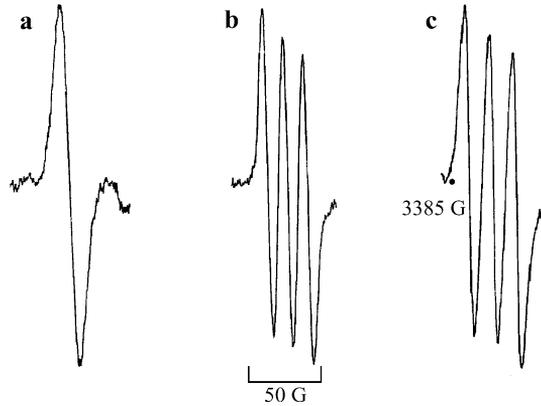
**Fig. 1.** ESR spectra of ROS in untreated wood (a) and wood treated (pH 3.0, 50 °C, 2 h) with laccase I (b) and laccase II (c).
