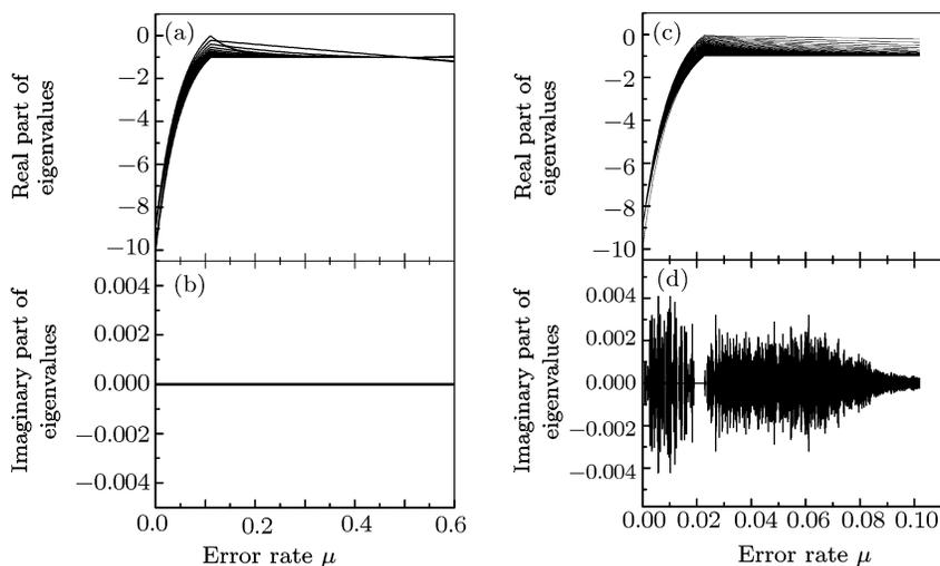
**Fig. 6** Eigenvalues of the Jacobian matrix with single-digit error rate for the Eigen model. The fitness landscape is the same as that in Fig. 1. (a) Real part of the eigenvalues with  $n = 20$ ; (b) Imaginary part of eigenvalues with  $n = 20$ ; (c) and (d) eigenvalues with  $n = 100$ .
