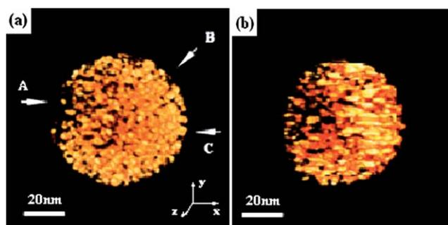
**Fig. 4** 3D reconstructed isosurface rendering viewing at  $0^\circ$  (a) and  $40^\circ$  (b) for the sphere as shown in the BF image of Fig. 3(d–f).
