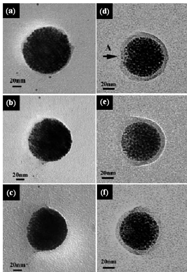
**Fig. 3** TEM images of a typical spherical aggregate with different tilt angles and cross-linking molecules, (a) 0°, octanedithiol, (b) +45°, octanedithiol, (c) +63.8°, octanedithiol, (d) 0°, biphenyldithiol, (e) –45°, biphenyldithiol and (f) +60°, biphenyldithiol.
