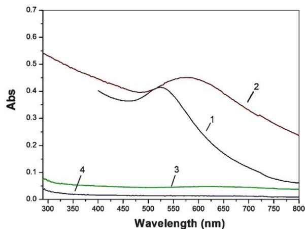
**Fig. 2** Optical absorption of the NPs dissolved in chloroform (plot 1), aggregates condensed from emulsion evaporation (plot 2), cross-linked aggregates by biphenyldithiols (plot 3) and octanedithiols (plot 4).
