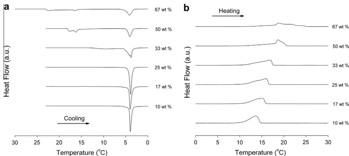
**Fig. 2.** DSC results of the  $\text{C}_{16}\text{mimCl}\text{-H}_2\text{O}$  systems upon cooling: (a) and subsequent heating and (b) scans at  $0.5^\circ\text{C}/\text{min}$ . Weight percentages of the surfactants in the mixtures are tagged to the respective curves.
