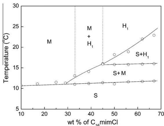
**Fig. 3.** Phase diagram of  $C_{16}mimCl-H_2O$  system. S (solid phase of  $C_{16}mimCl$ ),  $H_1$  (hexagonal phase), M (spherical micellar phase).
