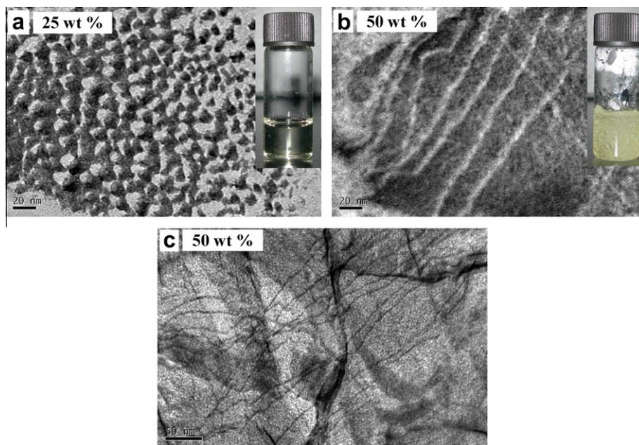
**Fig. 5.** (a) FFEM image of the 25 wt%  $C_{16}mimCl-H_2O$  sample at 30 °C. (b and c): FFEM images of the 50 wt%  $C_{16}mimCl-H_2O$  sample at 30 °C. The insets in (a and b) are the photographs of the two samples at 30 °C in glass vials.
