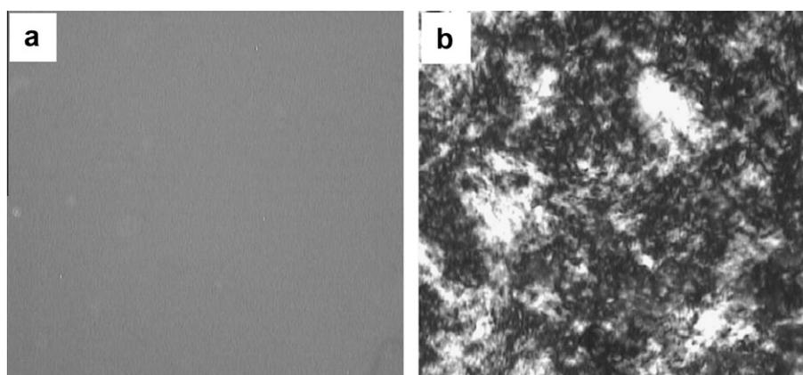
**Fig. 6.** POM images of  $C_{16}mimCl-H_2O$  mixtures at 30 °C. (a) 25 wt%, (b) 50 wt%.
