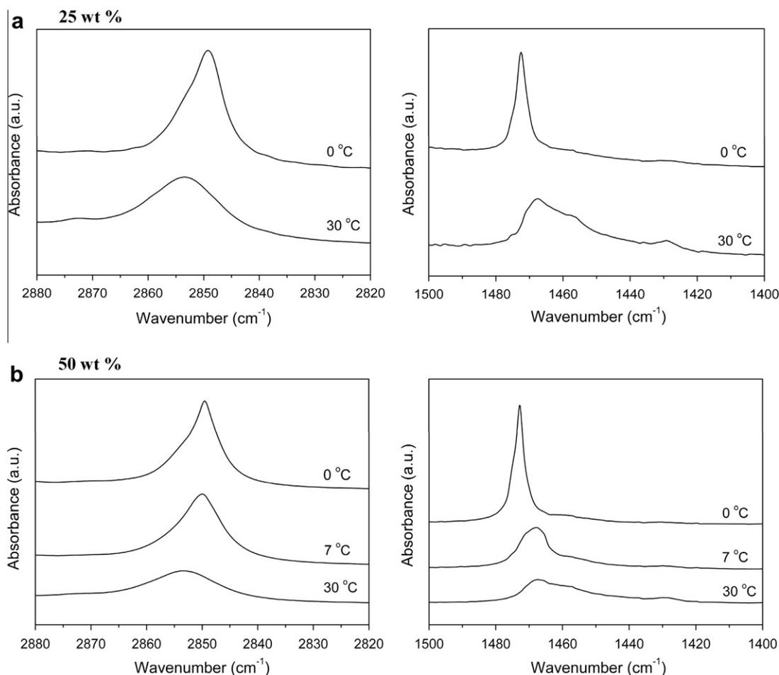
**Fig. 7.** FTIR spectra (2880–2820 and 1500–1400  $\text{cm}^{-1}$  regions) of  $\text{C}_{16}\text{mimCl-H}_2\text{O}$  at selected temperatures during cooling from 30 to 0  $^\circ\text{C}$  at 0.5  $^\circ\text{C}/\text{min}$ . (a) 25.0 wt%, (b) 50.0 wt%.
