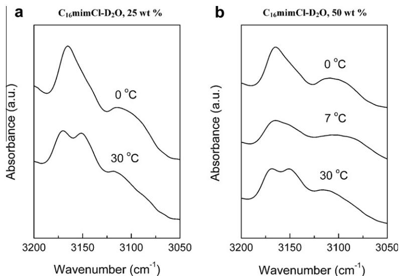
Fig. 8. FTIR spectra (3200–3050  $\text{cm}^{-1}$  region) of  $\text{C}_{16}\text{mimCl-D}_2\text{O}$  at selected temperatures during cooling from 30 to 0  $^\circ\text{C}$  at 0.5  $^\circ\text{C}/\text{min}$ . (a) 25.0 wt%, (b) 50.0 wt%.
