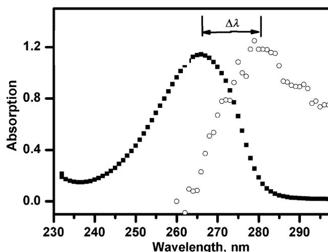
Figure 2. Normalized UV/Vis spectra of the salviatic acid A monomer (■) and Au@PEG3SA (○) in methanol.
