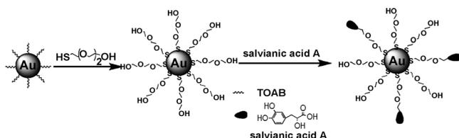
Scheme 1. Synthesis of salivianic acid A-functionalized AuNPs (Au@PEG3SA).
