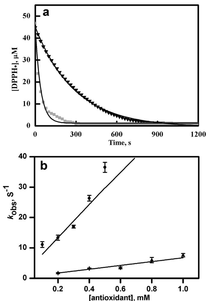
Figure 1. a) Decay of the DPPH radical in the presence of salviatic acid A (0.4 mM; black) and Au@PEG3SA (0.4 mM; gray). b) Plot of the pseudo-first-order rate constant ( $k_{\text{obs}}$ ) versus the concentration of Au@PEG3SA (●) and salviatic acid A (▲). Conditions: [DPPH] ( $45 \mu\text{M L}^{-1}$ ) in methanol.
