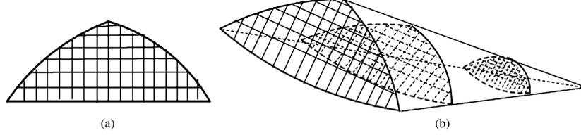
**Figure 2** The mesh segmentation in asymmetric unit. (a) The mesh segmentation in a given shell; (b) the mesh segmentation in different shells.
