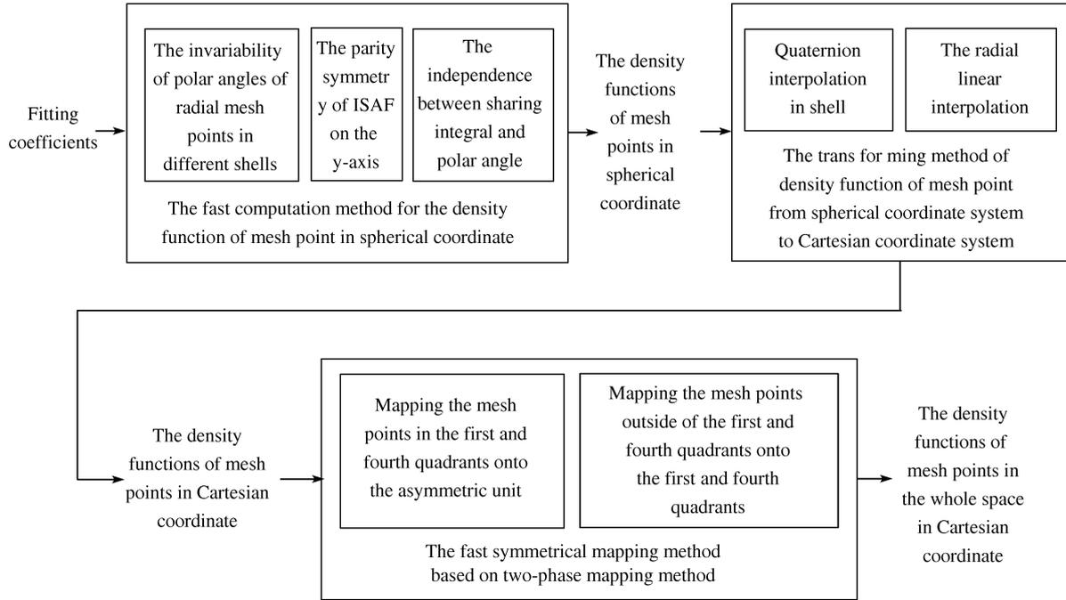
Figure 5 The fast calculation model of density function.
