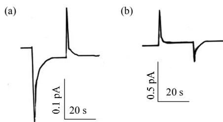
**Fig. 4 Photocurrent of dry photocell resulted from steel/cBRn film/Parafilm/ITO**
