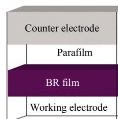
Fig. 1 Diagram of dry bacteriorhodopsin-based photocell
