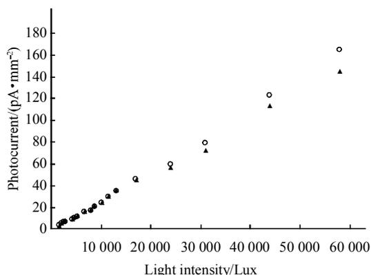
**Fig. 3 Photocurrent is linearly dependent on the change in the light intensity**
