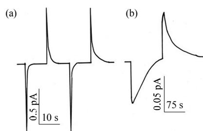
Fig. 2 Photocurrent of dry photocell resulted from ITO/cBRn film/Parafilm/steel
